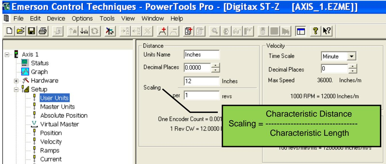
For example, if Dual Loop is enabled and you initiate an index distance of 12 inches and velocity of 24 inches per second, the pinch rolls would drive the material forward 12 inches as measured by the second encoder. With dual loop off, the motor would index the pinch rolls 12 \*26075/3000 inches, we simply need to divide out the ratio for the index distance (and velocity).
