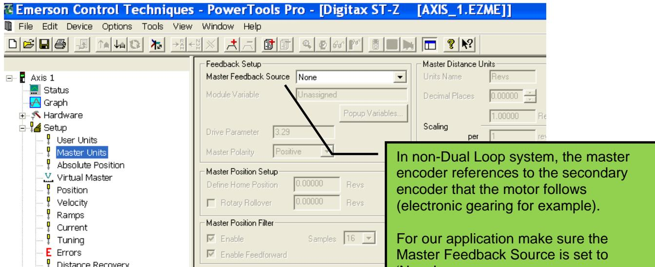
**In non-Dual Loop system, the master encoder references to the secondary encoder that the motor follows (electronic gearing for example).**
